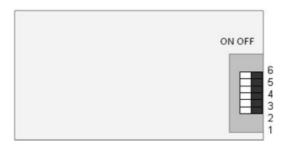
DIP Switched are located on the right hand side of the Printer after open the Top cover.
